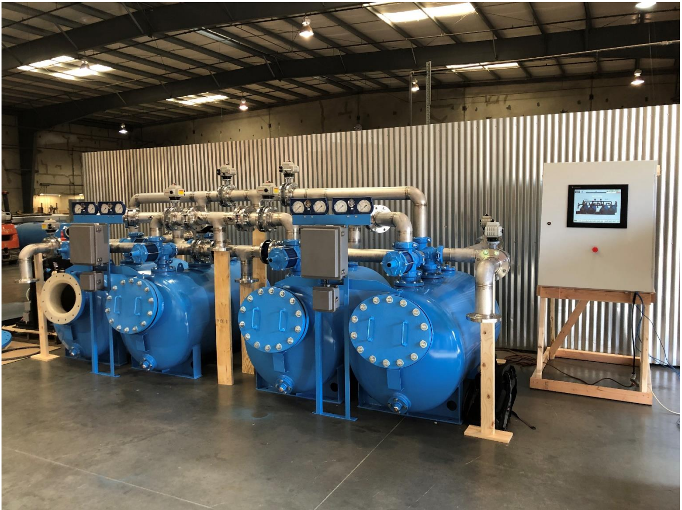
Photo 1: The filters were assembled for mechanical testing and final measurement. Representatives from DWA's Operations and Engineering Department inspected the filters.
