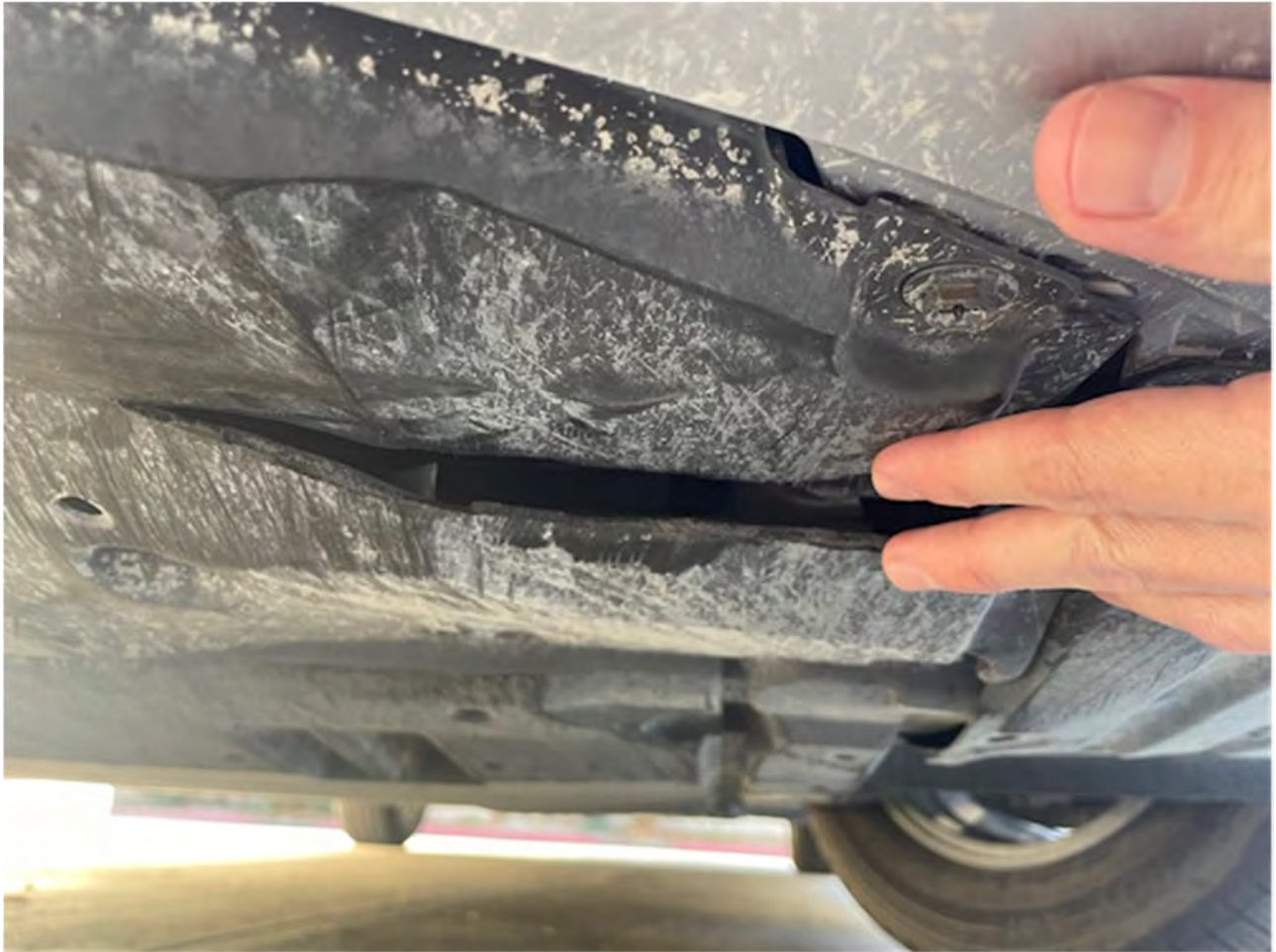
Photo 1 – Damage caused by cone to splash shield
