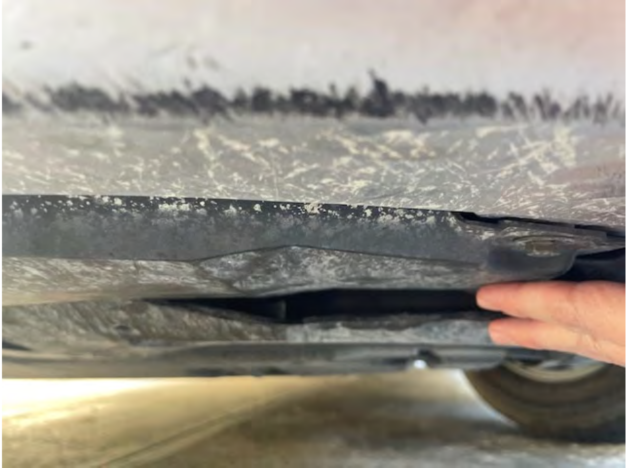
Photo 2 – Damage caused by cone to splash shield
