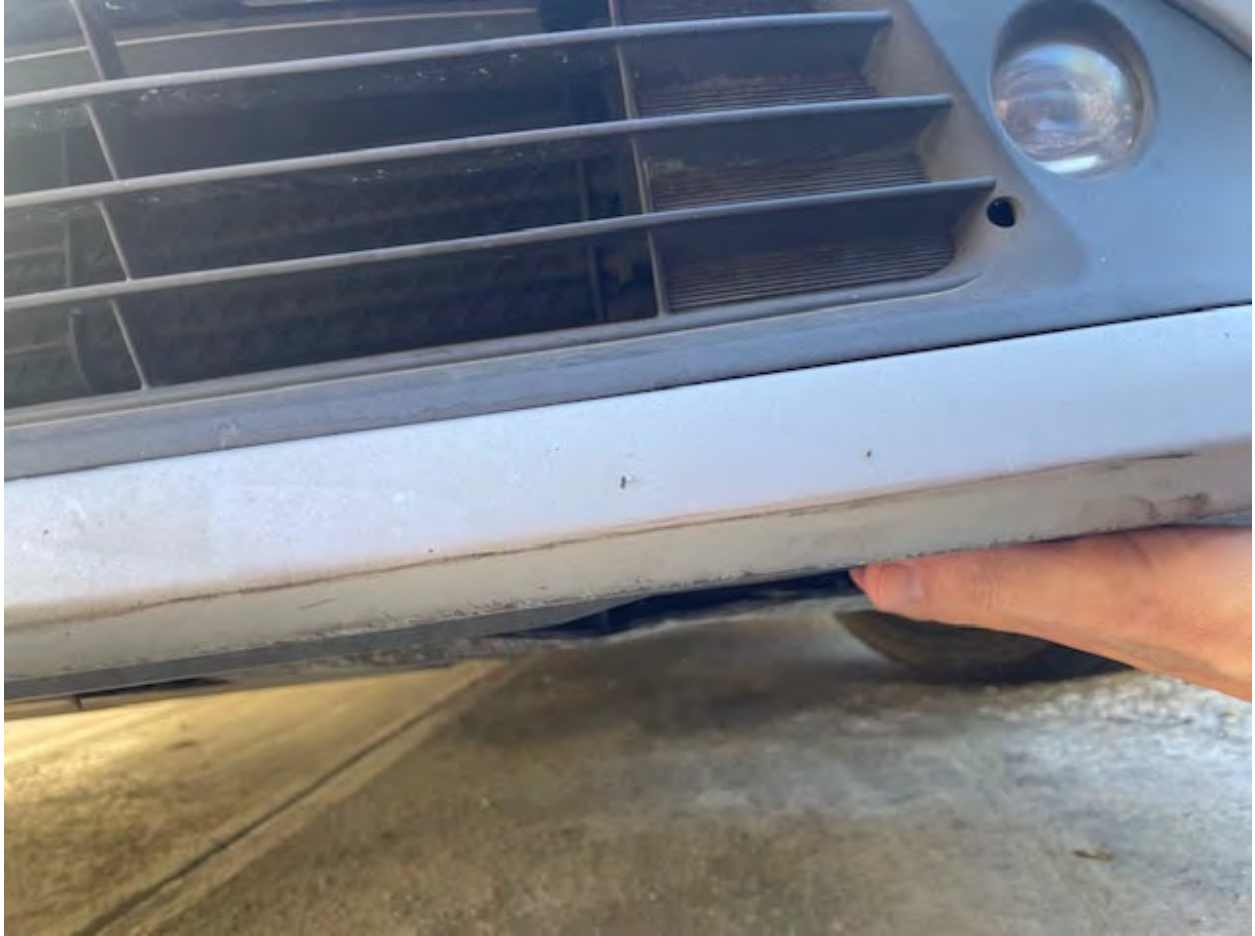
Photo 3 – Location where cone hit the splash shield right under “grill shutter” refer to video and second page of Toyota of the desert diagnostic/estimate.
