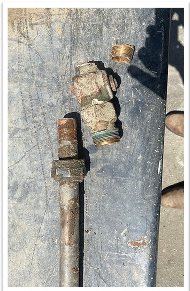
Damaged 1-inch corp stop and copper service line.
