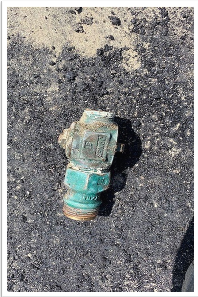
Damaged 1-inch corp stop and copper service line.
