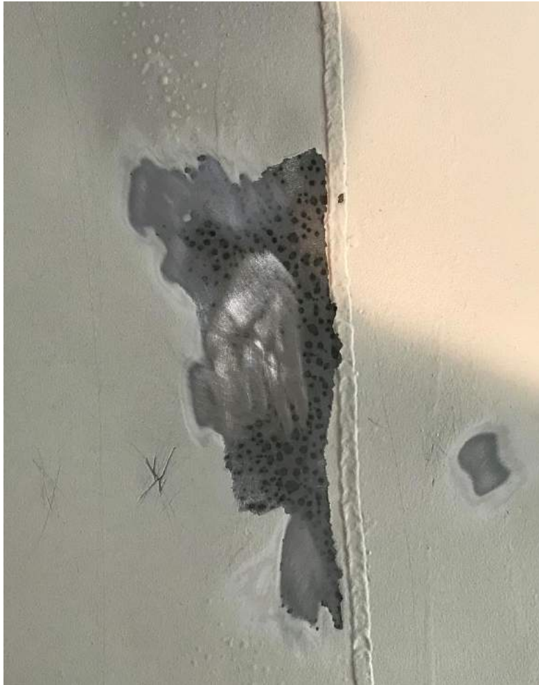
Photo 1: The black defects between the steel and the coating caused the paint to blister, which triggered the warranty repair.
