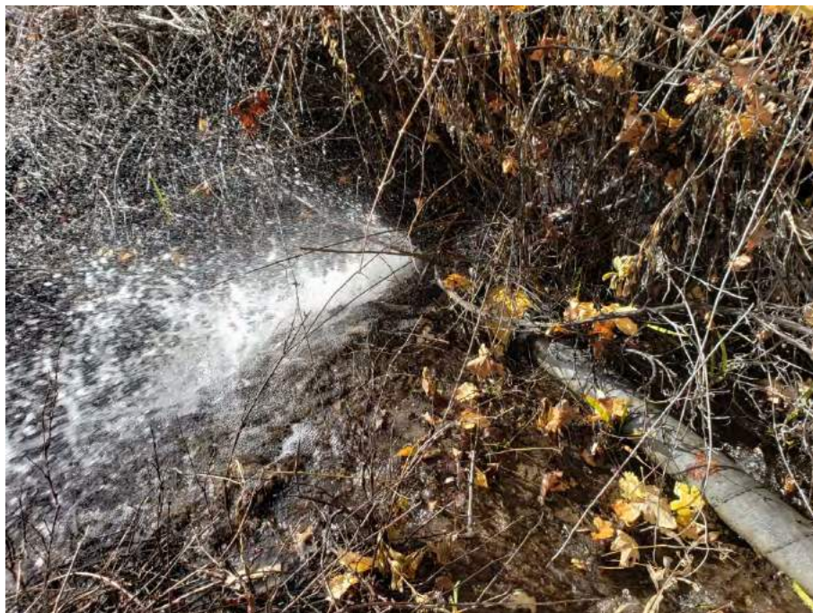
Photo 3: The Leak in the 4" Pipe
